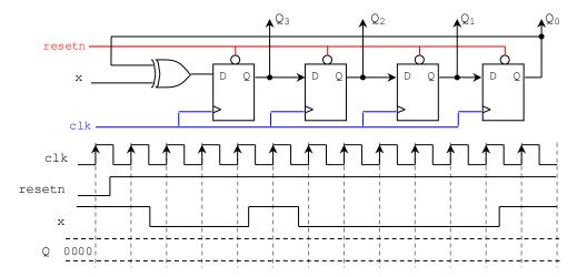
Complete the timing diagram of the circuit whose VHDL description is shown below. Also, get the excitation equation for q.
