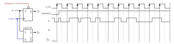
• Complete the timing diagram of the circuit shown below. (4 pts)
